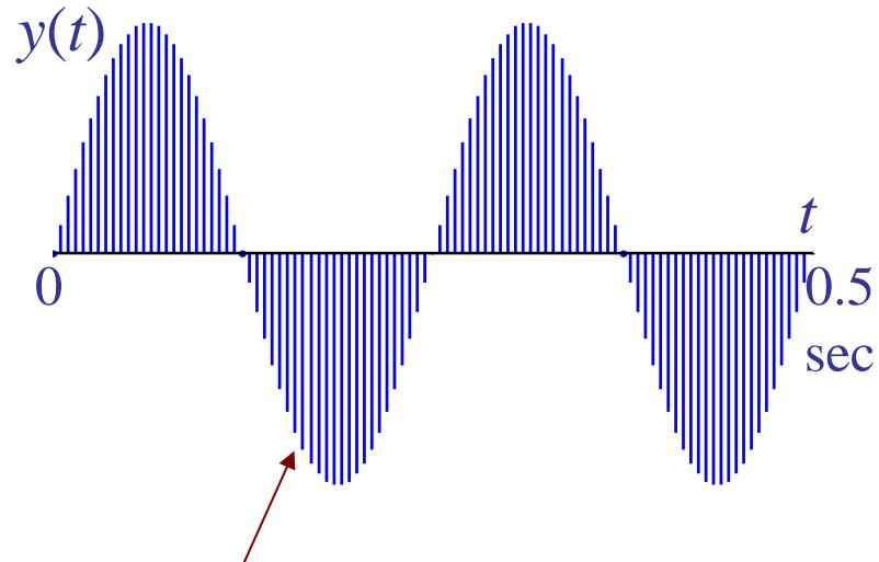
time samples are spaced at the default sampling interval  $T = 1/fs = 0.122$  msec
