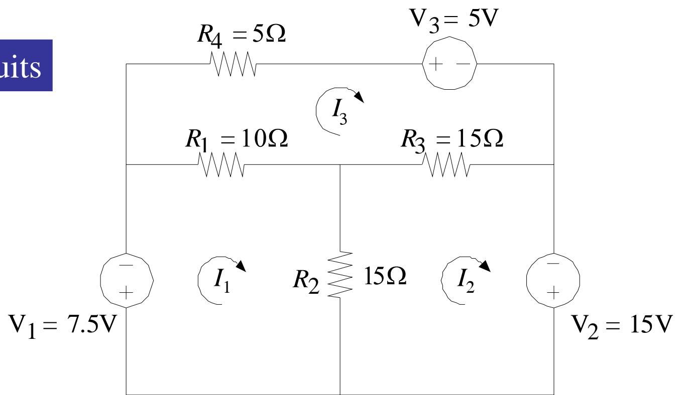
$$R_1(I_1 - I_3) + R_2(I_1 - I_2) + V_1 = 0$$
