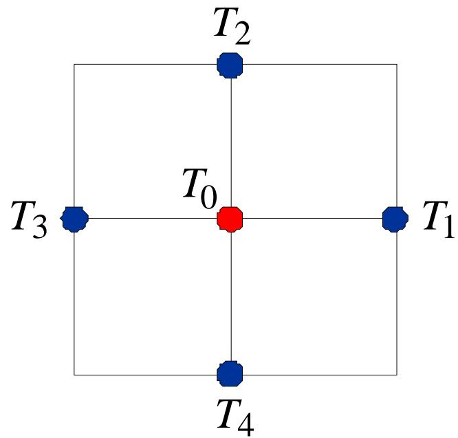
$$T_0 = \frac{1}{4} (T_1 + T_2 + T_3 + T_4)$$
